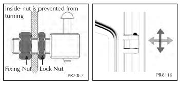
• Use a 19mm A/F spanner to loosen the fixing nuts
